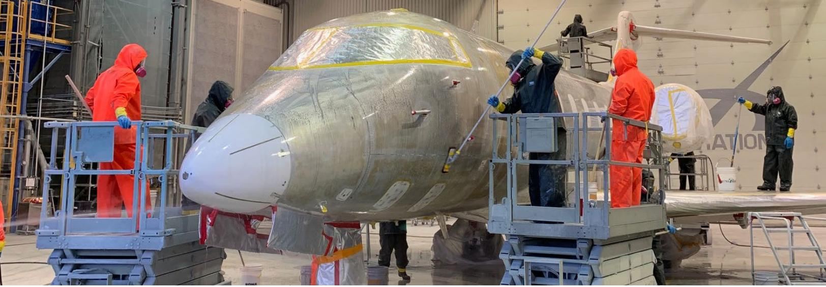
the old paint system and building it up with new filler primer and a topcoat. There are natural derivations in the manufacturer's assembly of the fuselage that a sand-and-paint can help smooth over," Kevin explains.
